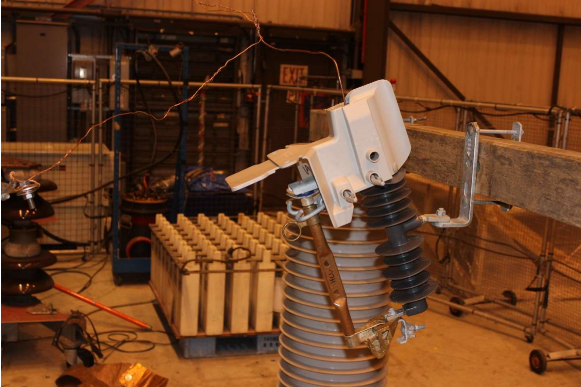
Figure 7. Lightning impulse withstand test setup
